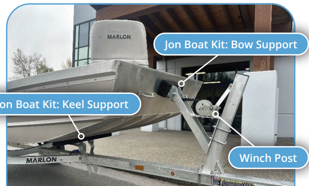
Jon Boat Kit Winch Post adjusted to support the bow of the boat, just above the bow's eye.
